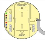
The 3X3-07 Model has three pairs of link pads: L1 L2 & L3 These are used to configure the switch for different functions. With reference to the individual scheme diagram, carefully abridge pads with solder only where indicated. Do this before installing in the guitar and avoid using excess solder. (Note: 7 interlinking wires are omitted in this view for clarity).
