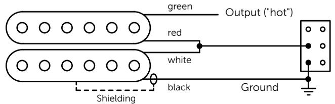
Parallel, out-of-phase and many other circuits are possible because of the pickup's four conductors.
