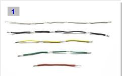
Prepare link wires by stripping insulation as shown above. Use multi-strand wire (equivalent gauge to pickup conductor wires).
