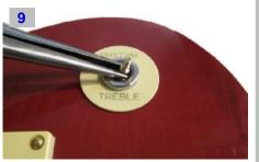
To remove/replace the toggle tip, move the toggle into position 2 and carefully grip it with long-nose pliars. Protect the finish to your guitar!
