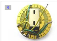
Solder the link wires onto the numbered pads as shown. Do not pre-tin the pads and avoid using excessive solder. Note ground connection. Casing is Stainless Steel and can not be soldered.
