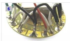
Some solder joints will span two pads - place the link wire between both pads and run the solder onto both pads evenly.
