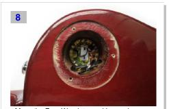
Move the Free-Way into position and secure with the nut and washer, replace back covers. Protect the finish to your guitar!
