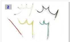
Shape the link wires by doubling over stripped sections, links should reach between the required pads without having excess wire.
