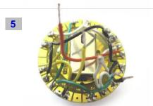
Link wire soldering completed - the wiring should not protrude beyond the switch perimeter to facilitate a clean install. Check for unwanted solder between pads - carefully scape to clear, if necessary.
