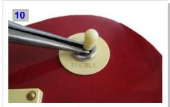
Screw the toggle tip tightly onto the threaded shaft - the pliars will prevent the shaft from rotating. The Free-Way tip is M3.5 size as standard.
