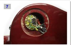
Before fixing in place, solder the guitar wiring to the link wiring and insulate connections. Protect the finish to your guitar!
