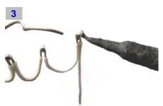
Tin the link wires using multicore solder as shown above - this will simplify soldering to the pads.
