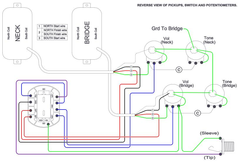
Tin the solder pads prior to soldering the wires.
